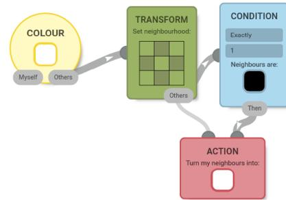
Fig. 5. A Transform node in use to specify a restricted neighborhood to be reused. The Colour node has two properties.
