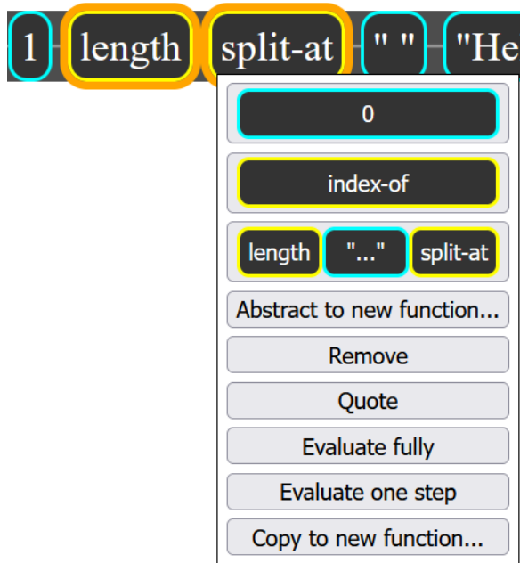
Figure 2: A (trimmed) menu of splice options for a selected subsequence. The selected terms have a thick orange highlight, around the yellow border of the two operation terms. The value terms, with blue border, are not selected and will not be replaced by the selected menu operation.
