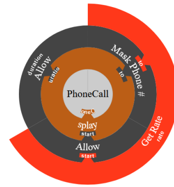
Figure 4. A program in a radial view, representing one of the suggested use cases for the view, filtering and masking information for data governance purposes. Values move outwards from the centre, being processed at each layer.
